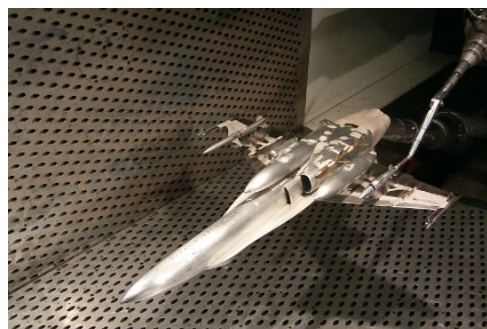
Figure 3: CTS Wind Tunnel Test.
