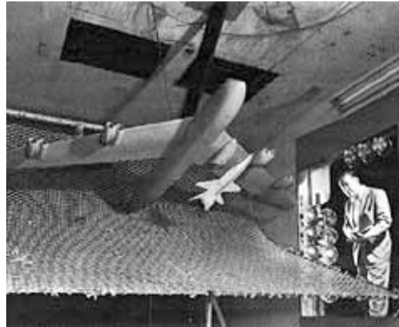
Figure 2: X-15/B-52 Drop Test.
